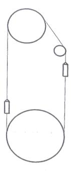
Determine for a nominal winding cycle the available stopping distance – as required by Directive C2 – from the stopping point, where the emergency brake would come on if the speed controller fails at the end of the full speed zone. Ensure that the emergency deceleration would not cause slip at the driving sheave wheel. Assume a friction force of 10 kN for each conveyance.
